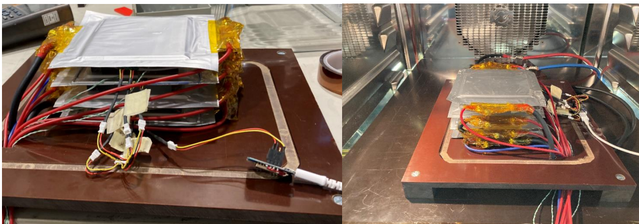
Figure 13: Emulation of a four-cell battery module; Left: A Four cells daisy chain stack of the Custom Cells integrated with the CMU; Right: The Four cells stack inserted in a controlled climate chamber for measurements
