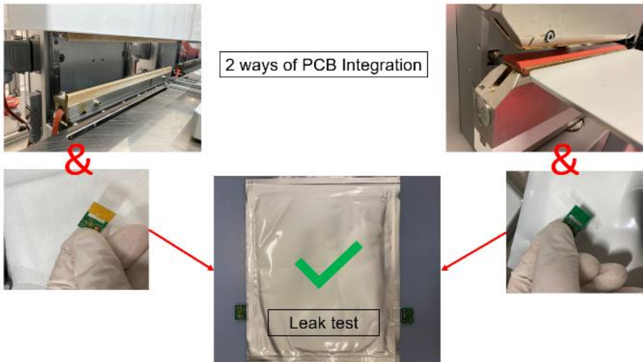
Figure 6: Two possible ways of PCB integration at AIT using different sealing equipment and PCB design. Rigid steel sealing bars combined with flexible PCB layout (left side) and flexible sealing bars with rigid PCB layout (right side)
