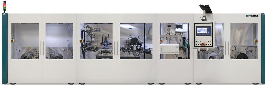
Figure 7 Electrode Notching Machine, MANZ AG [Manz.com](http://Manz.com)
